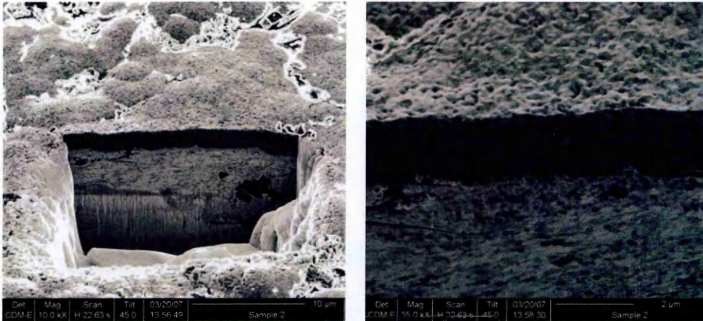
Figure 4-2: FIB Sections of 'Matt Metallic' Electrodeposited Platinum Black Metallic
