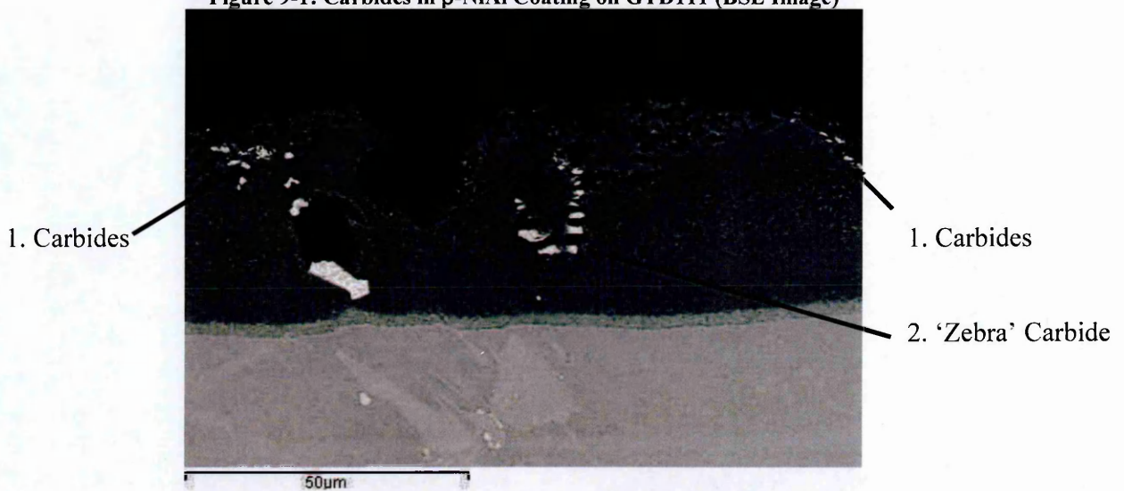
Figure 9-2: Carbides in \beta -NiAl Coating on GTD111 (BSE Image) (2)
