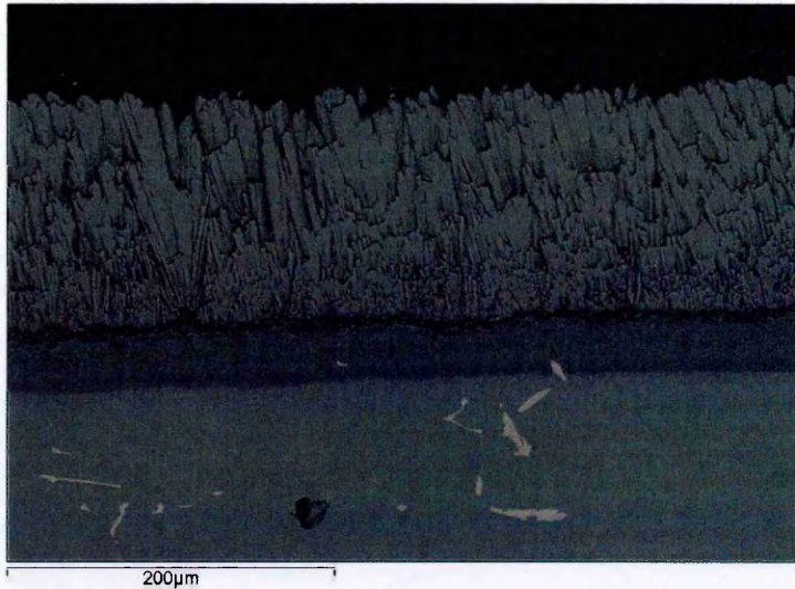
Figure 5-4: Photomicrograph of ILAl Heat Treated with ICON followed by Application of TBC (BSE Image)
