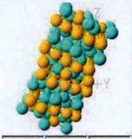
Figure 8-10: Structure of NiTa (Pearson hR13) 172
