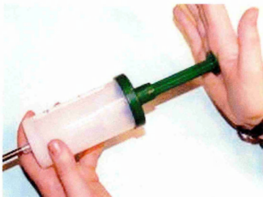
Figure 3. Bio-VOC sampler (Markes International) attached to a Tenax-Carbotrap tube.
