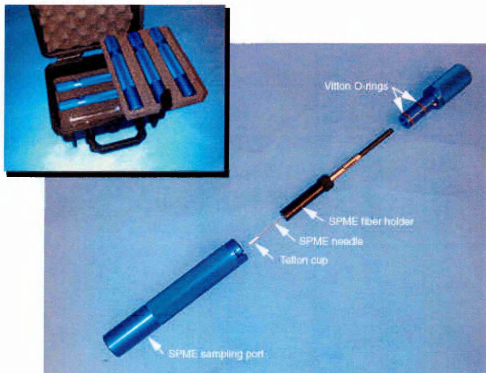
Figure 2. Photograph of a SPME holder (taken from http://www-cms.llnl.gov/s-t/solid_phase.html (Lawrence Livermore))
