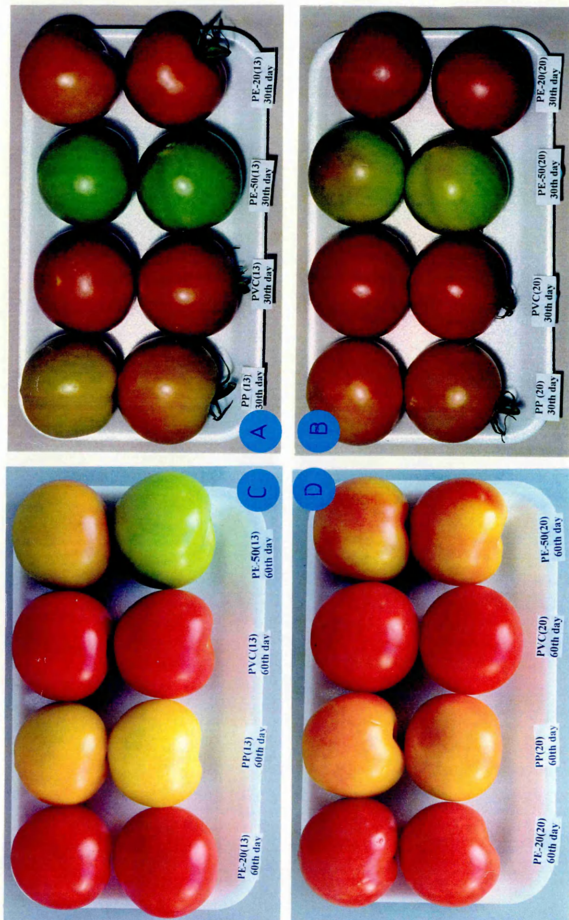
Plate 6.1. Some tomatoes stored in various MAP films. (A) at 13°C for 30 days; (B) at 20°C for 30 days; (C) at 13°C for 60 days and (D) at 20°C for 60 days
