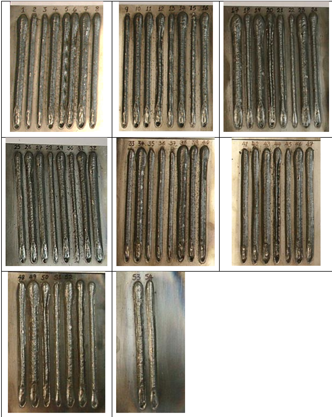
Figure 3-12 Surface appearance of Tandem-GMAW deposited weld beads
