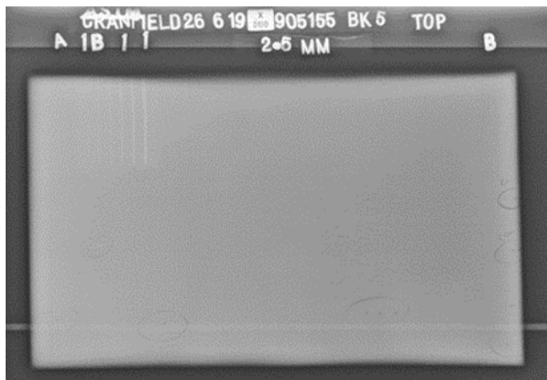
Figure 5-8 X-ray radiograph image of WAAM test block, showing sound internal structure of the weld metal
