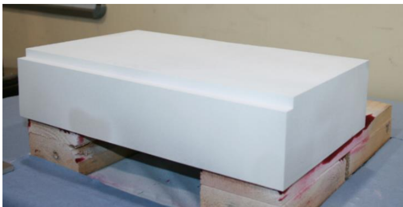
Figure 4-7 Dye penetrant test on WAAM block
