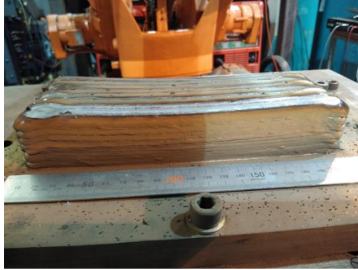
(a) Completed WAAM block, showing quality of side surface
