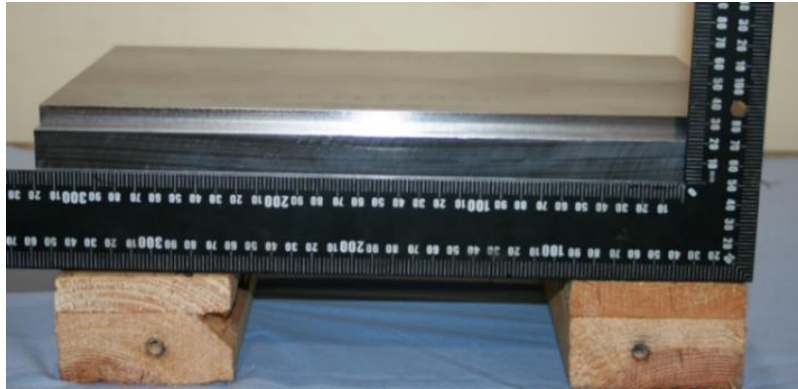
Figure 4-6 Machined WAAM block, measuring (320 x 210 x 75) mm
