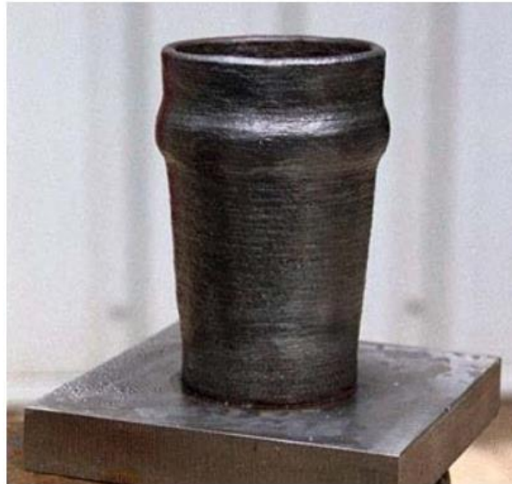
Figure 2-18 WAAM beer mug produced using GMAW process. Ribeiro, F. (1998b)
