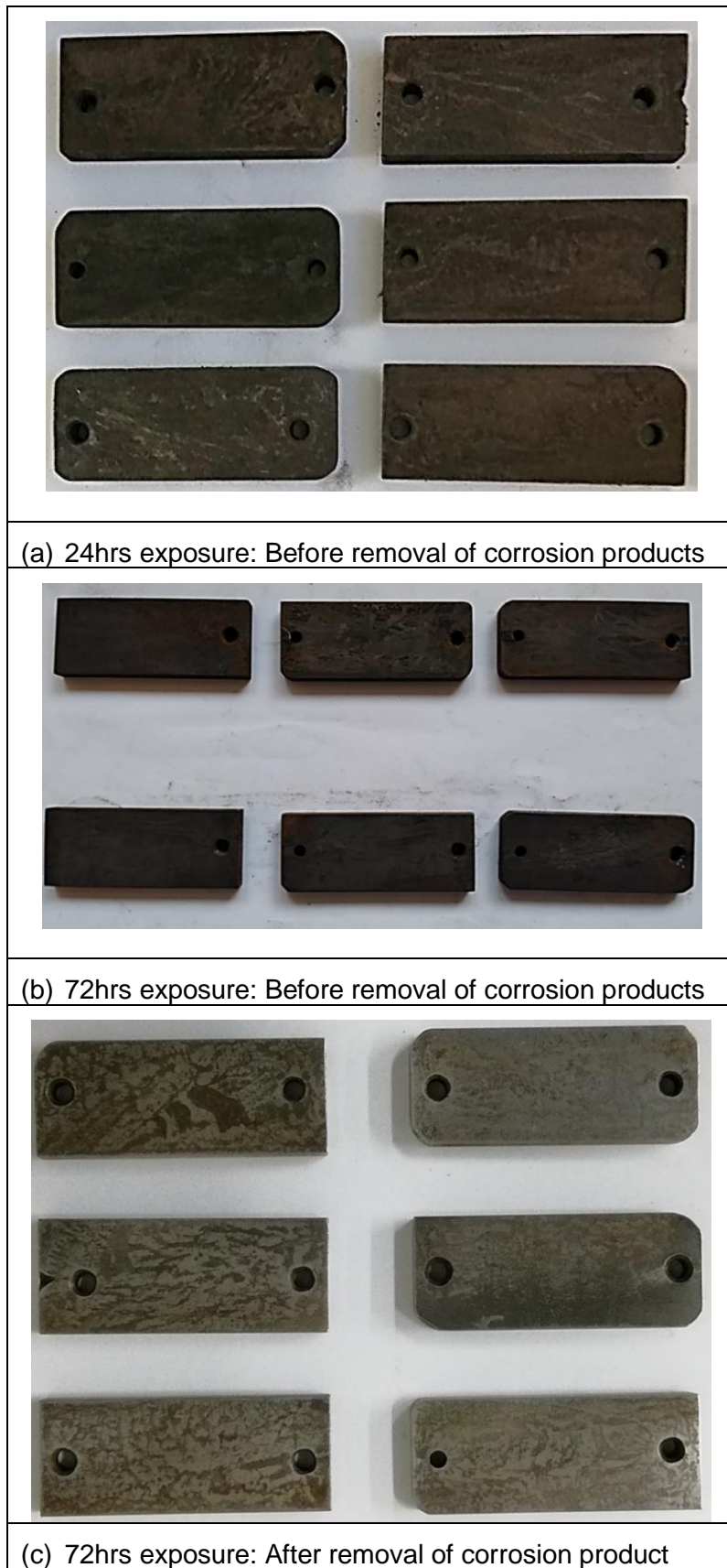
Figure 6-3 Surface appearance of samples after exposure to corrosion
