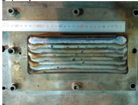
(b) Completed WAAM block, showing quality of top surface
