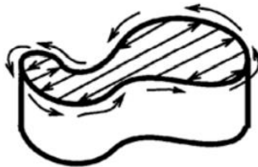
Figure 2-26 Deposition of perimeter and layer filling with the use of raster path in LENS process (Hensinger, D. M. et al., 2000)
