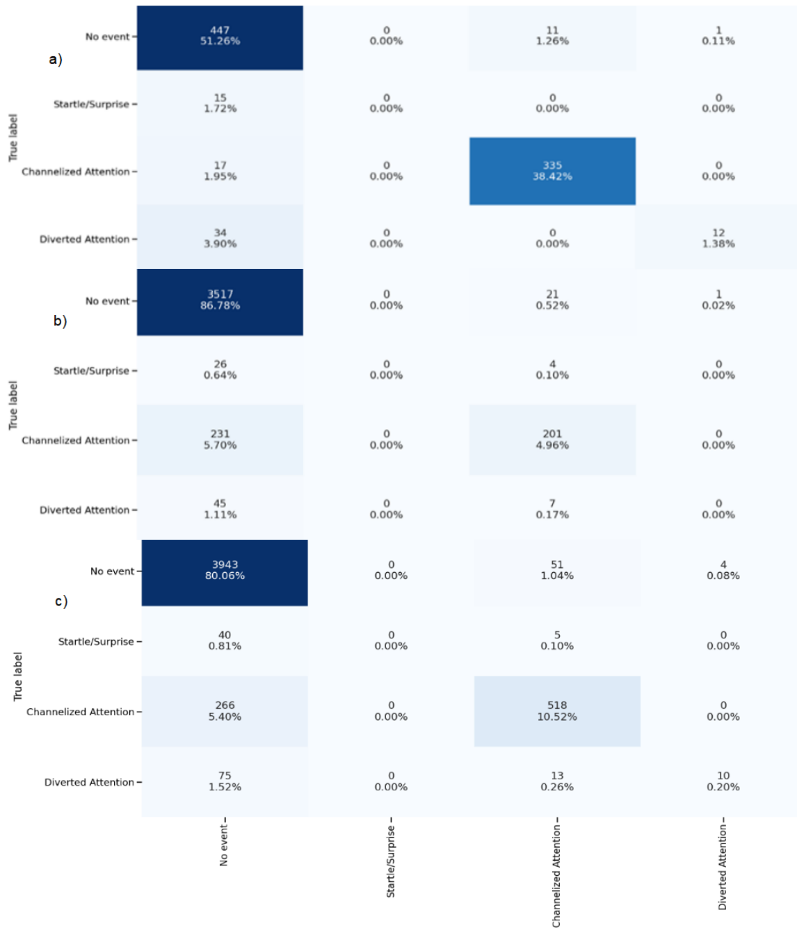
Figure 4: SVM model's confusion matrix for unprocessed data collected from a pilot in a) non-flight environment, b) flight environment, and c) merged non-flight and flight environments
