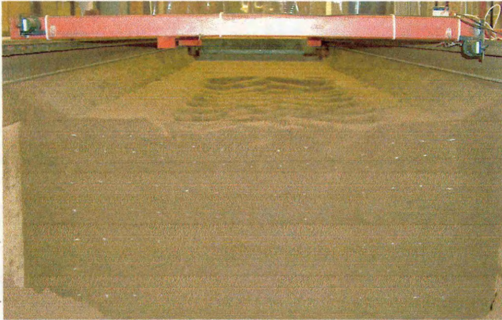
Figure 8: 2 nd Replication of vertical cut for the 800 mm section width tire run at 1.25 bar and loaded to 10.5 t
