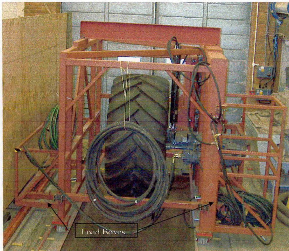
Figure 16: Single wheel tester over soil bin with a 900 mm section width tire inside
