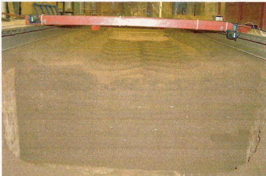
Figure 23: Vertical cut through soil with points of talcum powder when the 900/10.5/1.9 had passed.
