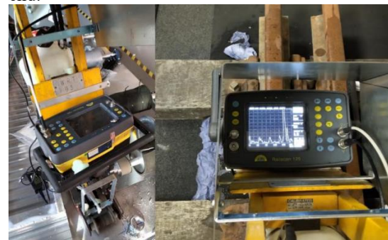
Fig. 2. Rail walking stick, probe and flaw detector of UT system.
