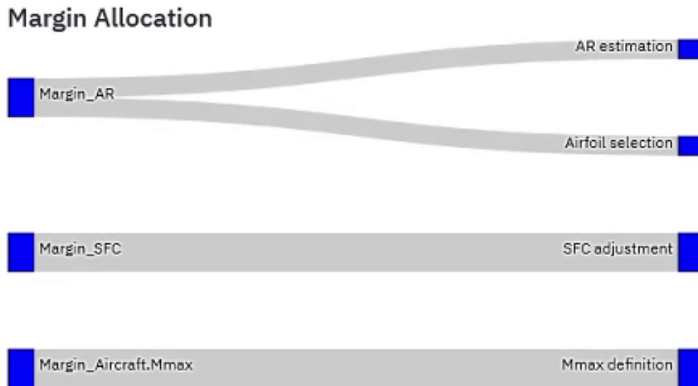
Figure 6.22: Updated Sankey diagram of margin-assumption dependencies corresponding to Use Case 1 (Software prototype tool)
