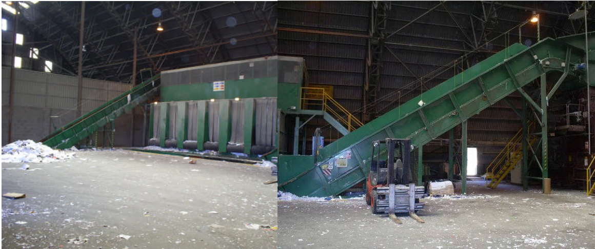
Figure 12: Sort line (on the left) and conveyor belt A of zone 2 going through to the baler (on the right).
