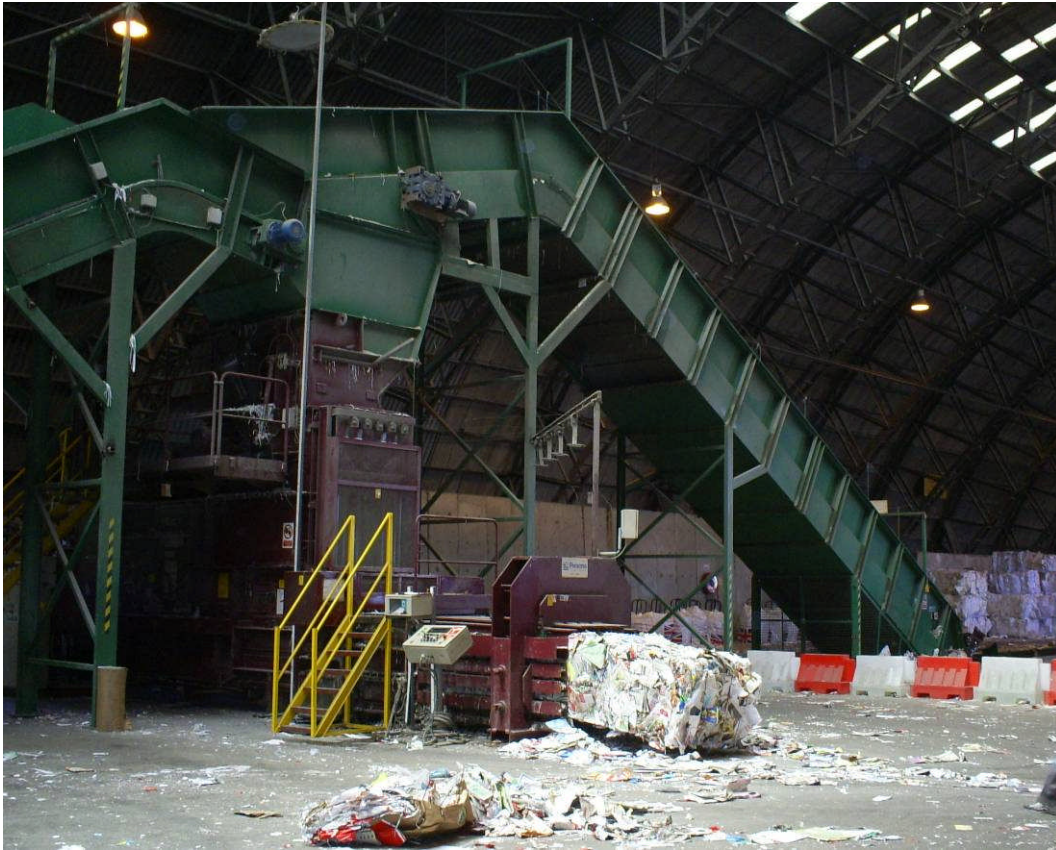
Figure 14: Conveyor belt B of zone 3 going through to the baler and bales coming out of the baler.
