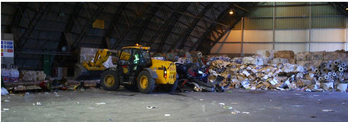
Figure 13: Operator loading papers, plastics or cardboards onto conveyor belt B (zone 3).
