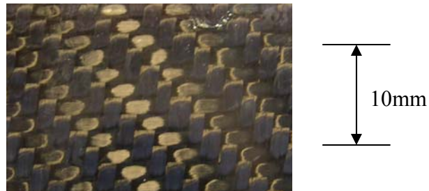
Figure 2-31: 2x2 Twill IM9-2035 material used in the nosecone of the BAR 006
