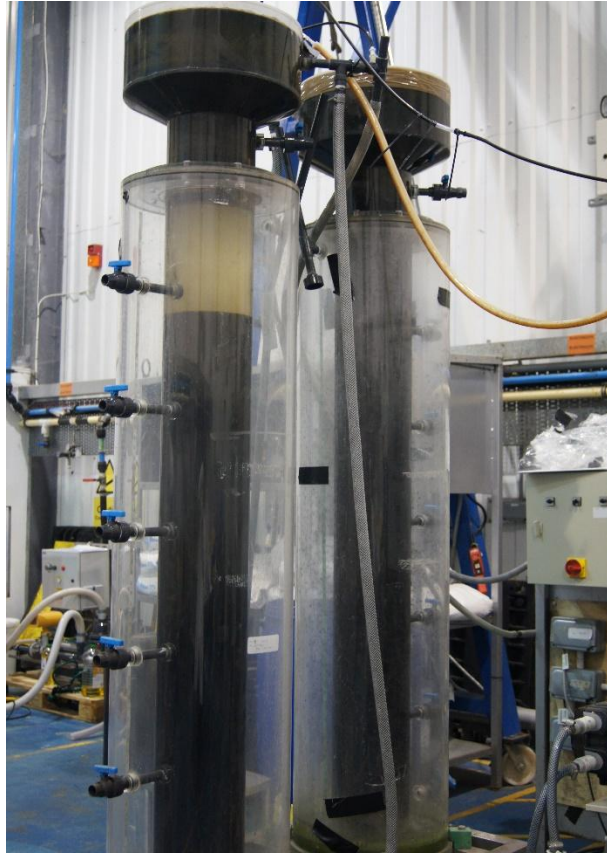
Figure A- 1. 70 L upflow anaerobic sludge blanket (UASB) reactors with granular and flocculent inoculum biomass (Chapter 3 and Chapter 4).
