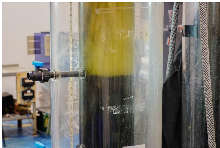
Figure A- 2. Sludge blanket in granular UASB reactor.
