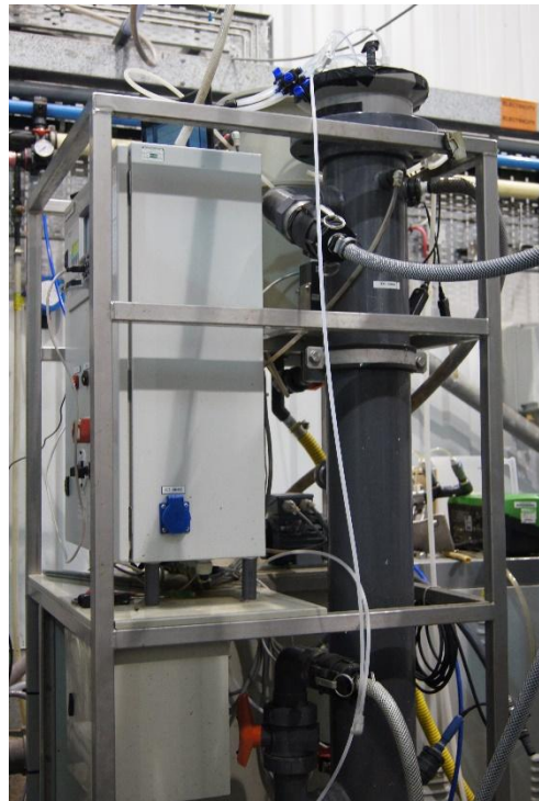
Figure A- 4. 42.5 L granular UASB reactor coupled with 30 L membrane tank (Chapter 5 and Chapter 6).
