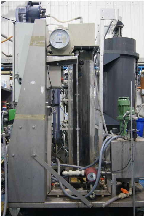
Figure A- 4. 42.5 L granular UASB reactor coupled with 30 L membrane tank (Chapter 5 and Chapter 6).
