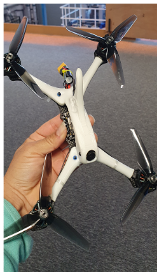
Figure 7: Non-Symmetrical Structure - NSY.
