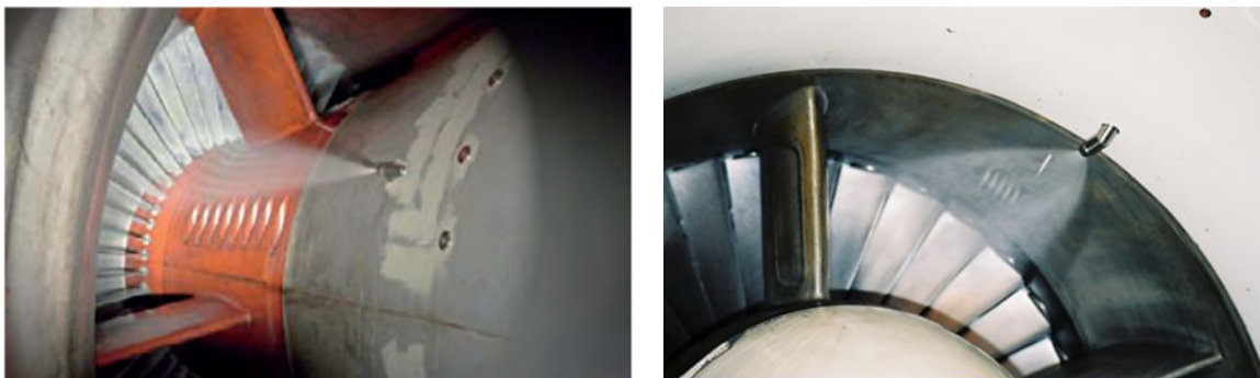
Figure 3 Online compressor washing arrangements – Left: nozzle on the bellmouth [10] and Right: nozzle on the plenum [11]
