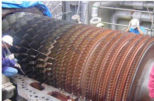
Figure 1 Front stage fouling of a multi-stage compressor [9]
