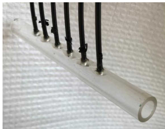
Figure 2: Typical Acrylic burn tube, this tube has a 7 mm inner diameter and 100 mm length.
