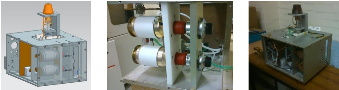
Figure 39. Plasma torch in UG model (left), fixed match structure (middle) and Plasma torch
