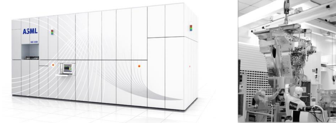
Figure 4. TWINSKAN NXE3300B (Left); completely integrated illuminator during preparation for shipment (Right)
