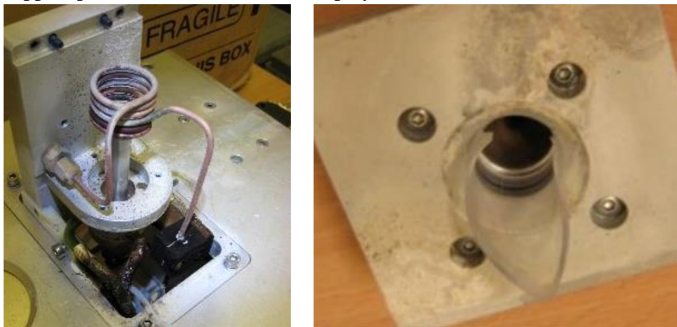
Figure 28. Damage of Helical coil and De-lava nozzle support images. [30]
