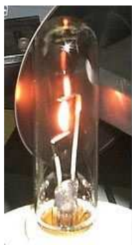
Figure 62: The tungsten strip filament lamp used for the absolute light intensity calibration. The filament itself is a strip of tungsten presenting a flat 4mm by 6 mm polished section on its centre. It is held by 2 metallic pins within an evacuated glass cylinder.
