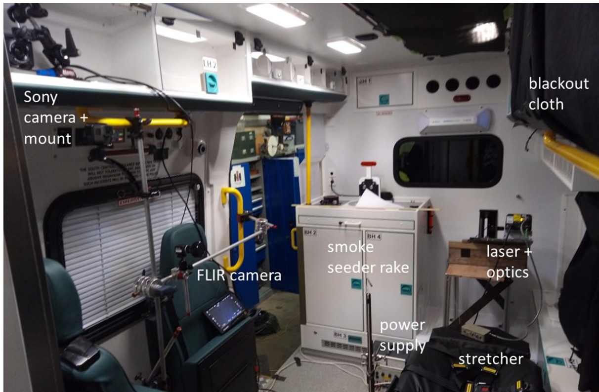
Figure 2 – General layout of lab equipment in ambulance
