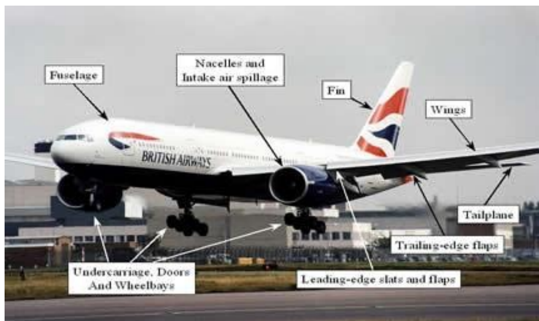
FIGURE 2.6: Airframe noise sources
