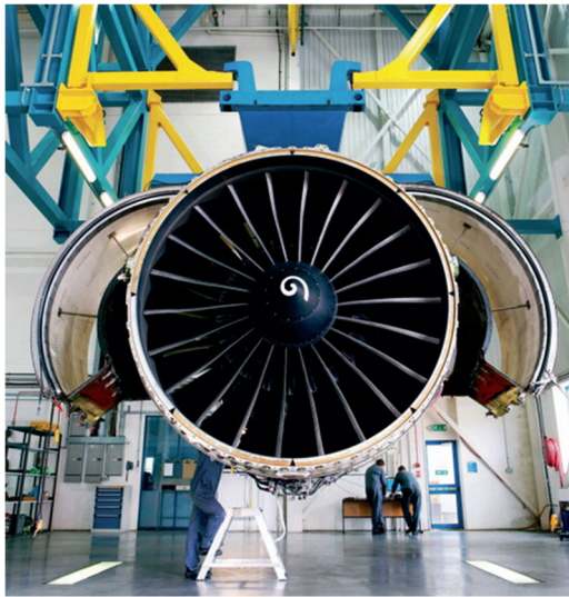
FIGURE 1 A GE90 engine with 22 carbon fiber composite fan blades. Reproduced with permission. 2 Copyright 2012, Elsevier
