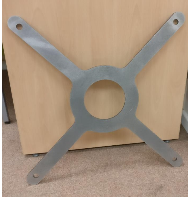
Figure 8 Steel line spacer. The anchor or buoy was tied to the spacer through the large hole in the centre, whilst the ropes connecting the frames were run through the small holes on each arm.
