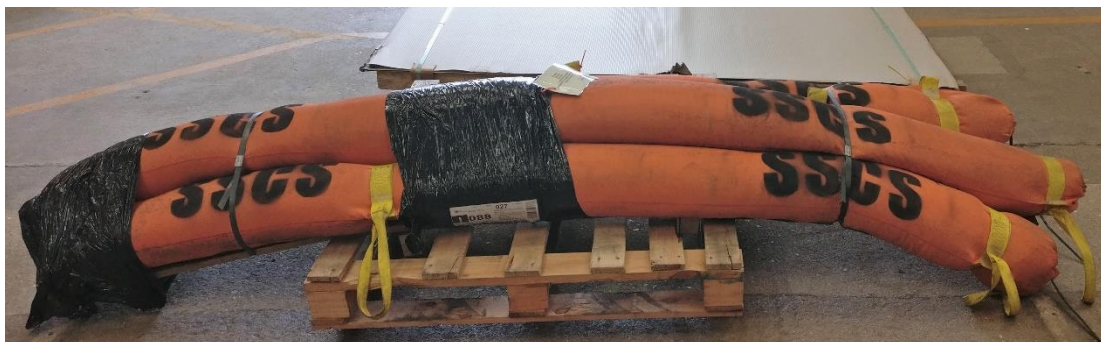
Figure 7 Aggregate filled tubes used to anchor the mooring systems.
