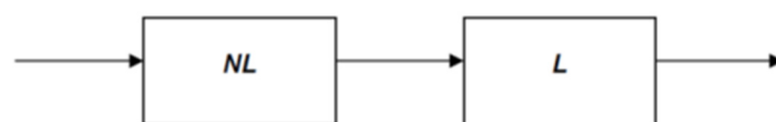
Figure 4. Control structure showing the sequence of the application of the Wiener approach to calculating the nonlinear condition followed by the linear conditions for the valve response time.
