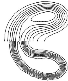
FIG. 9. Helium bubble shape in terms of volume fraction isovalues. Comparison between DG^3 (top half) and DG^1 (bottom half) resolution. [Adapted with permission from E. Franquet and V. Perrier, “Runge-Kutta discontinuous Galerkin method for the approximation of Baer and Nunziato type multiphase models,” J. Comput. Phys. 231 , 4096–4141 (2012). Copyright 2012 Elsevier Ltd.]
