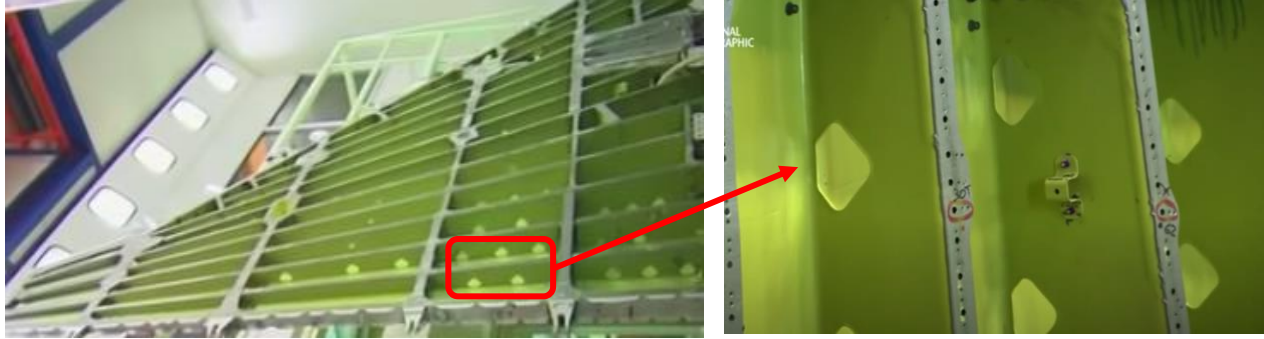
Figure 1. Typhoon multi spar wing panel structure and fuel transfer holes (Geographic, 2012).
