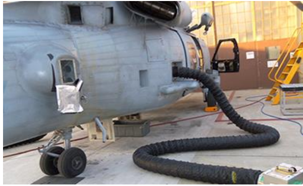
(a) Fuel tank ventilation.
