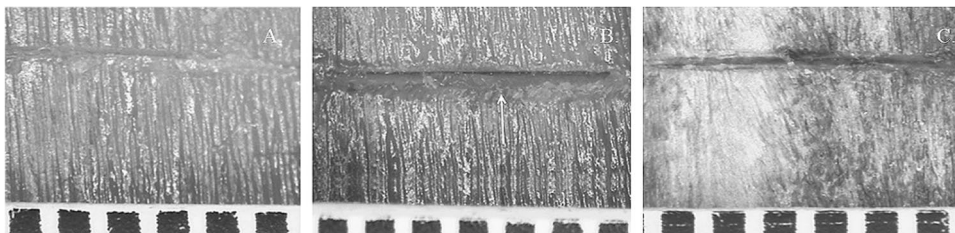
Fig. 3 A view of a cut mark inflicted by A a non-serrated blade, cutting edge width 1.78 mm; B a coarse-serrated blade, cutting edge width 2.45 mm (the white arrow indicates a raised edge); and C a fine-serrated blade, cutting edge width 2.31 mm; scale in mm
