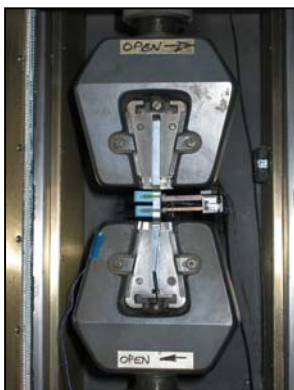
Fig. 3.1.4.3. Dynamic strain gauge extensometer mounted on the dog bone specimen
