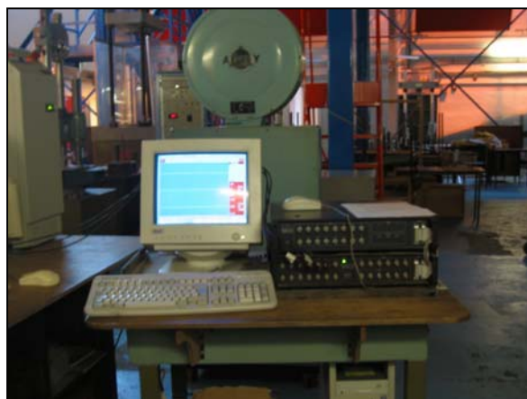
Fig. 3.1.5.1. Data Logger with maximal sampling frequency of 12 kHz/channel
