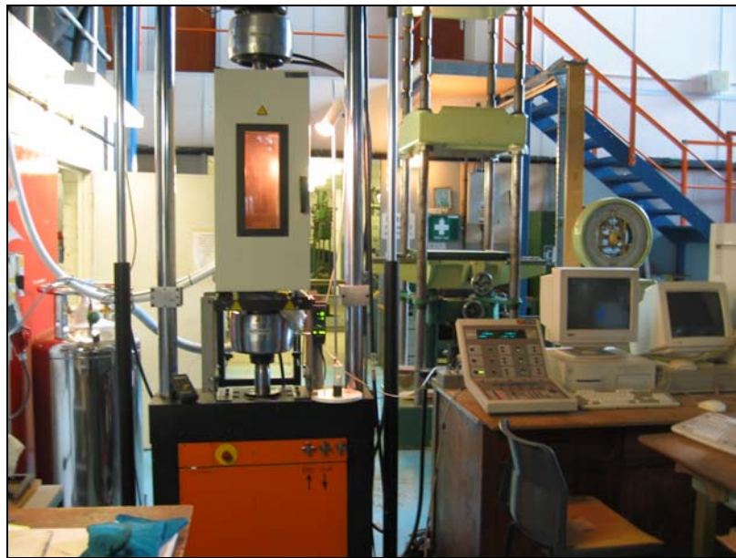
Fig. 3.1.4.2. 100 KN Servo Hydraulic Fatigue Machine with maximal steady-state velocity of 80 mm/s
