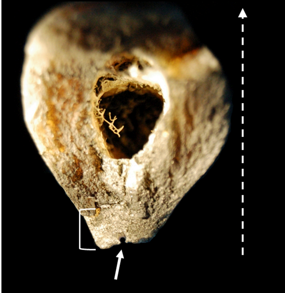
Figure 3: Crack origin at the site of a nutrient foramen opening; solid arrow indicates the nutrient foramen opening on a posterior human femur, bracket indicates the mirror zone, and the dashed arrow indicates the direction of crack propagation.
