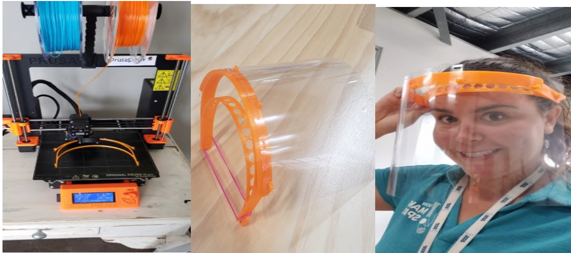
Figure 2: 3D printed head-ring, a rubber band, and a soft plexiglass shield
