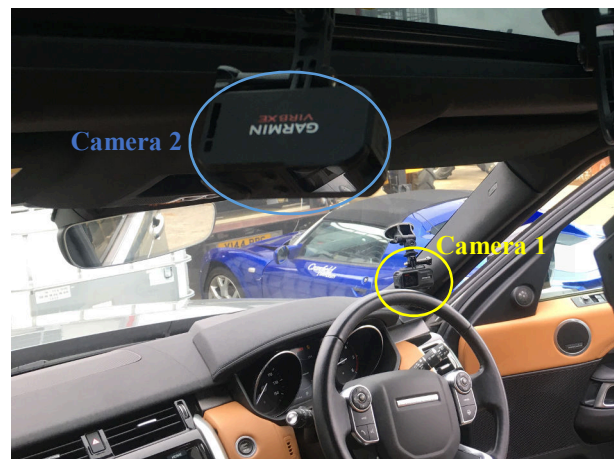
Fig. 4. Cameras inside the vehicle. Locations have been highlighted by different colours.
