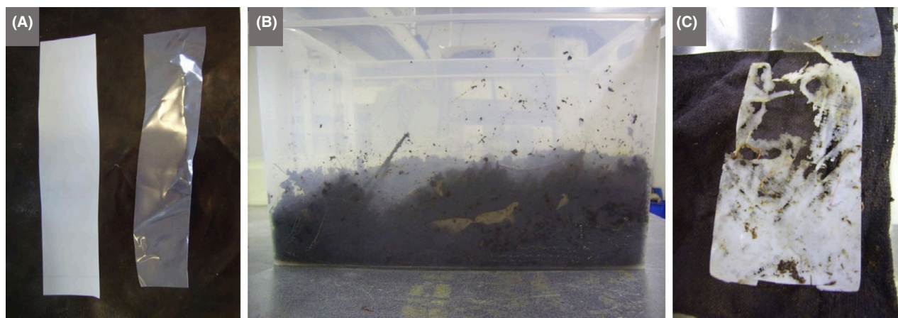
Fig. 8. Bioplastic degradation in compost
