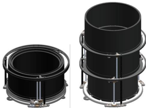
Fig. 1 Telescope structure in stowed and deployed configuration
