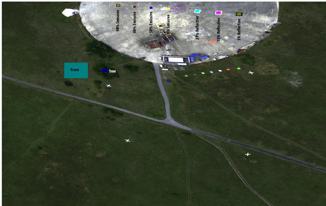
Figure 5.3: Location and reflectivity of calibration panels planted within the Ground Truth Selene scene [10].
