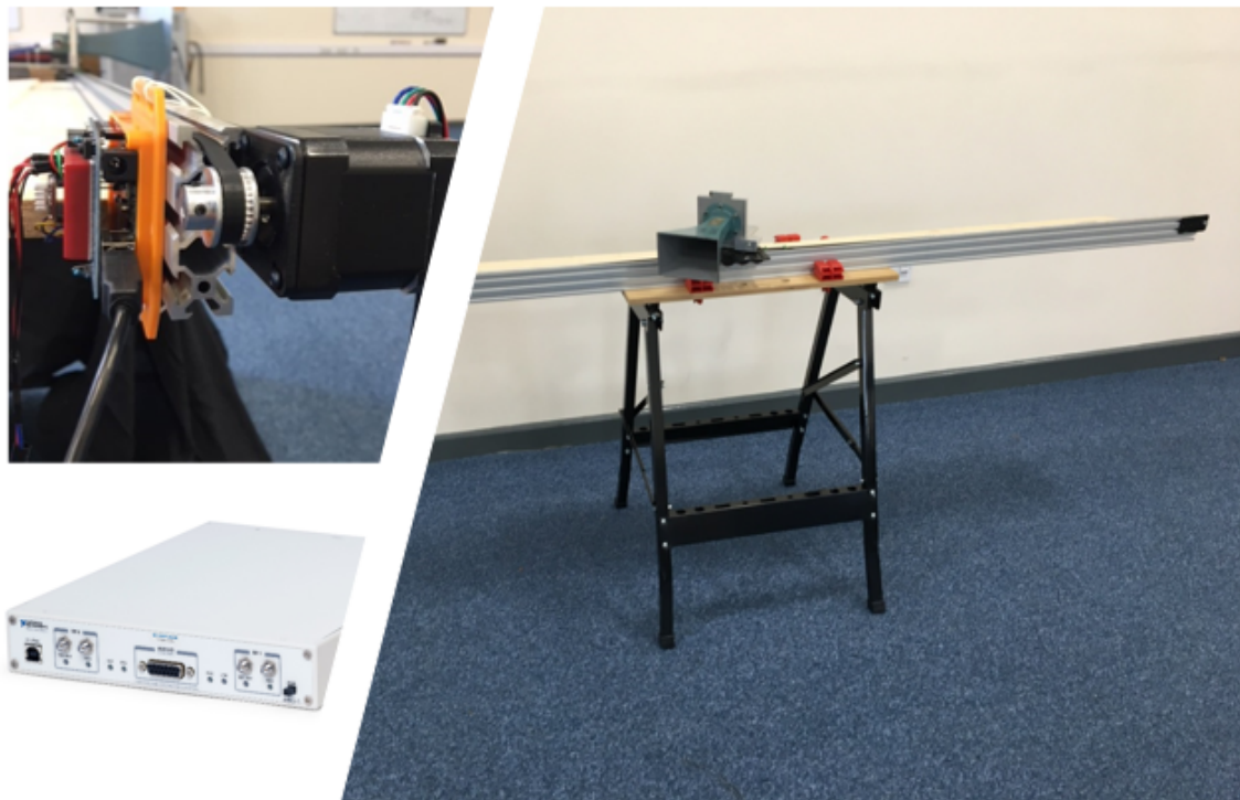
Figure 4.1: Constructed DBS Rail
