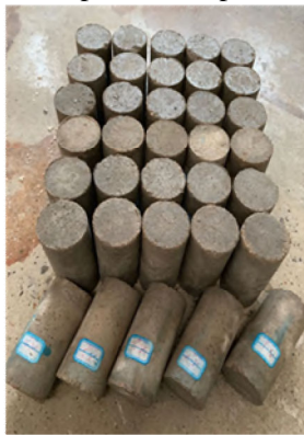
Fig. 6 Part of the cement mortar test samples.
