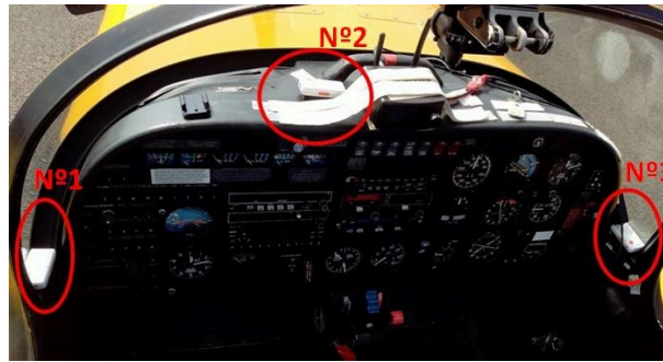
Figure 7: Position of the three accelerometers inside the aircraft's cockpit.
