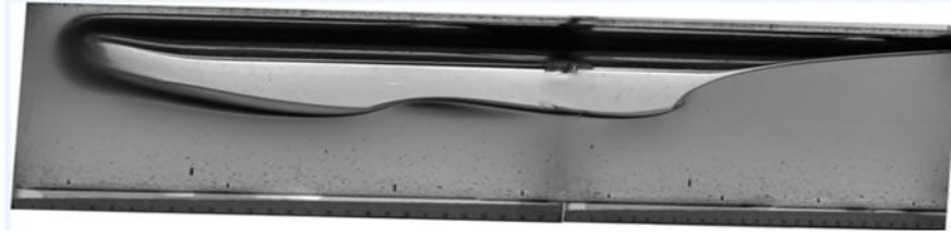
(b) 2.5degree_Vso = 0.21 m/s, Lb/D=3.324, Fr_d=0.4176 , VOLgas = 0.002246 m 3 . Original image size: Height, 31.2 mm, and Width, 115.7 mm. Scaled dimension: Height, 90% and Width, 100%
