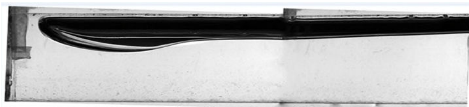
(a) 160 cP_0.099 m ID pipe_1degree, L_b/D = 10.90 , Fr_d = 0.4052 , VOL_{gas} = 0.004493 m 3 , (LTT). Original image size: Height, 32.9 mm, and Width, 123.1 mm. Scaled dimension: Height, 84% and Width, 100%
