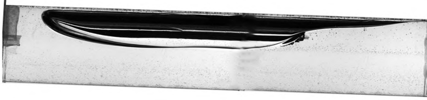
(b) 160 cP_0.099 m ID pipe_2.5degree, Lb/D=5.05 , Fr_d=0.4272 , VOL_{gas} = 0.002996 \text{ m}^3 , (STT). Original image size: Height, 67.9 mm, and Width, 223.4 mm. Scaled dimension: Height, 41% and Width, 53%
