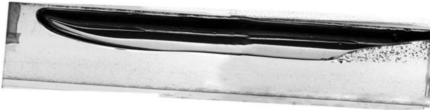
(c) 160 cP_0.099 m ID pipe_5degree, Lb/D=7.07 , Fr_d=0.4394 , VOL_{gas} = 0.004493 \text{ m}^3 , (STwtB). Original image size: Height, 39 mm, and Width, 131.8 mm. Scaled dimension: Height, 80% and Width, 91%
