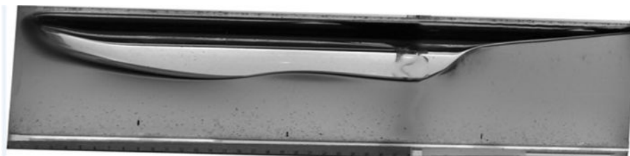
(a) 2.5degree_ V_{so} = 0.11 \text{ m/s} , Lb/D=3.89 , Fr_d=0.4176 , VOL_{gas} = 0.002246 \text{ m}^3 . Original image size: Height, 31 mm, and Width, 120.8 mm. Scaled dimension: Height, 93% and Width, 100%
