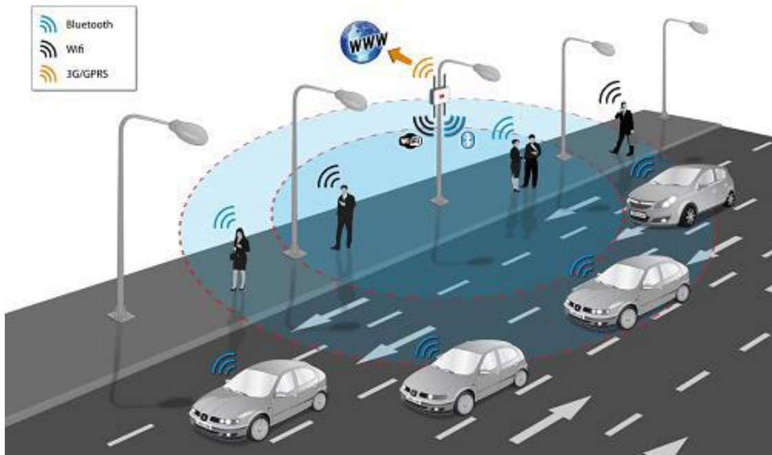
Figure 12. Using electric poles for connectivity between users and vehicles through Wi-fi and Bluetooth (Pal & Pali, 2018).
