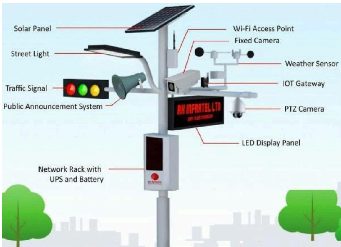
Figure 13. How an electric pole is made smart as an IoT gateway (Pal & Pali, 2018).
