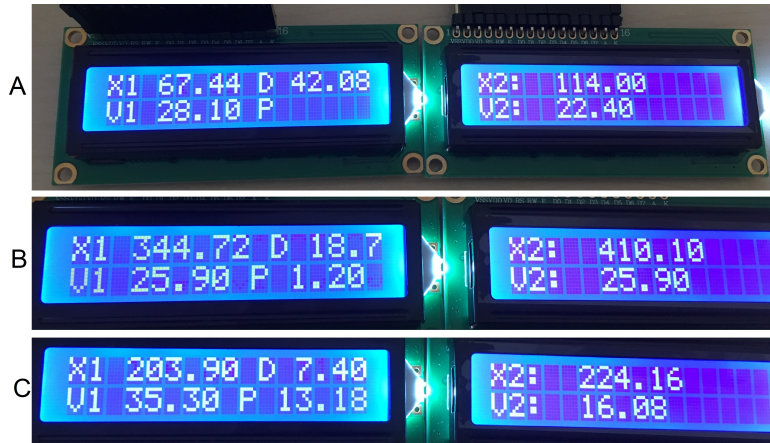
Figure 36: Raspberry Pi displays, respectively, during the approach, cruising freely, platooning and overtake. As the EV, denoted as 1, approaches, it executes the algorithm as presented in Fig. 18 in Section 4.1. The OV may reject it, but accepts, as the payment offsets the cost, and executes the requested speed profile.
