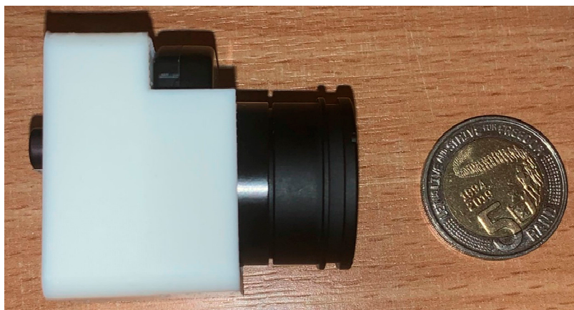
Figure 2. FLIR Boson In a 3D printed case next to a coin for scale, the camera weighs around 7.5 g.
