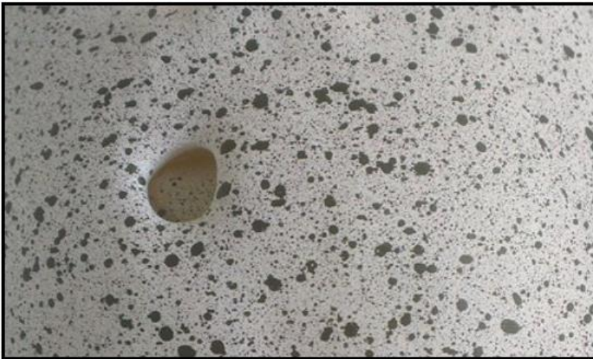
Figure 2 - Typical speckle pattern, exemplified using a model with an excision to show the brain simulant within.
