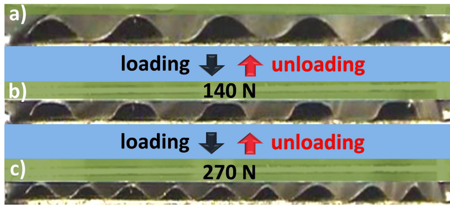
Fig. 2. Side-view snapshots of the shaped MG foil during use as a linear wave spring. (a) Free-standing pre-shaped MG foil. (b) Elastic deformation at the maximum load when still functioning as conventional wave spring. (c) The undulatory behaviour in which further loading leads to elastic multiplication of the number of arcs in the waveform and to an increase in the load capacity.
