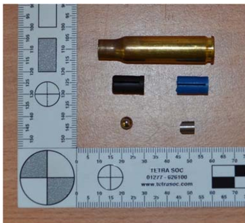
Fig. 2 Cartridge case (top), sabots (middle), BB (bottom left) and CN FSP (bottom right)
