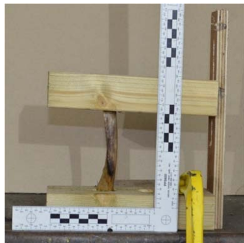
Fig. 3 Custom-made wooden frame used to hold each rib specimen
