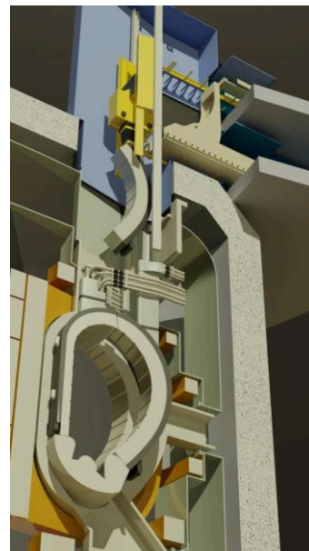
Fig. 1: Vertical port blanket extraction handling scheme
