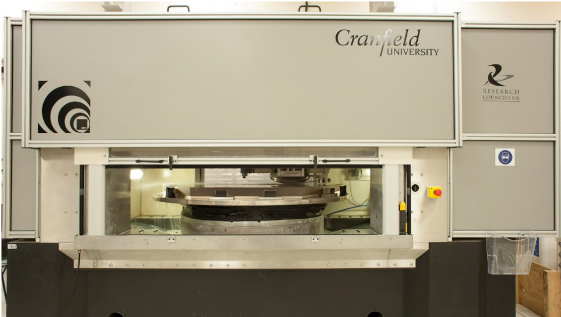
Figure 8-13: Machining ESO E-ELT segment on BoX
