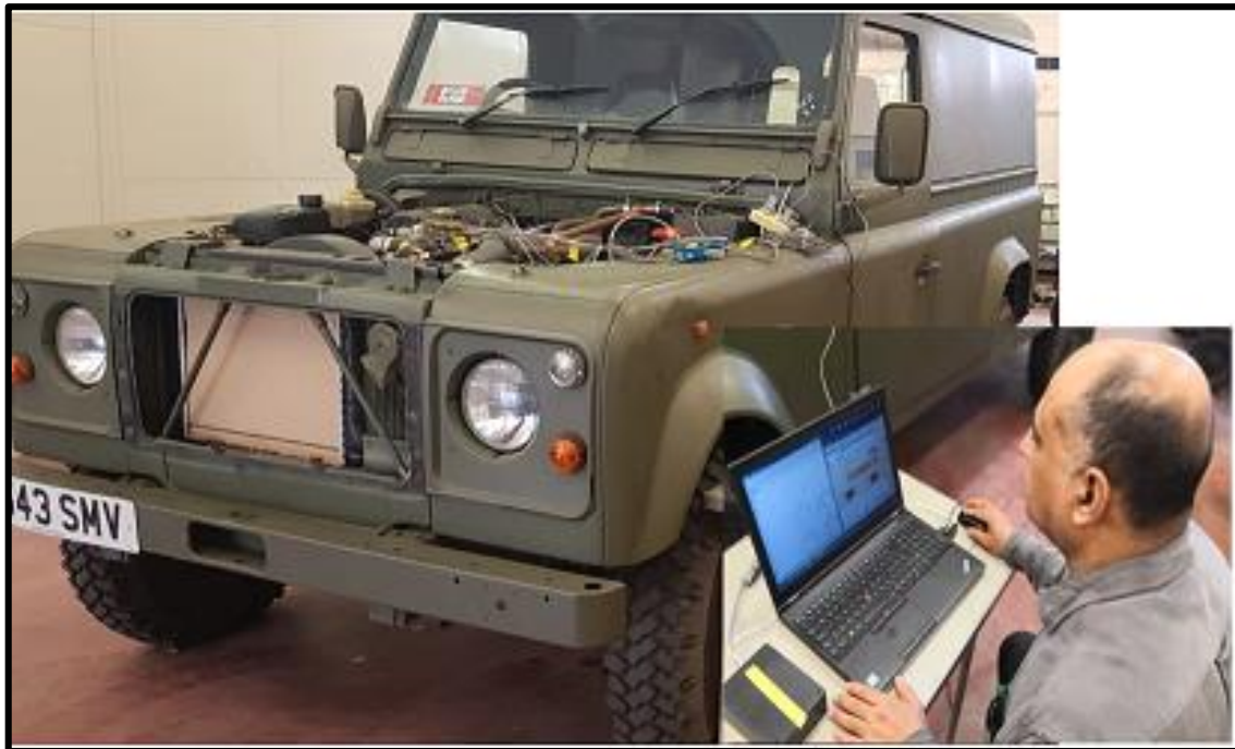
Figure 3.16 Land Rover110 test platform with instrumented cooling system HUMS.
