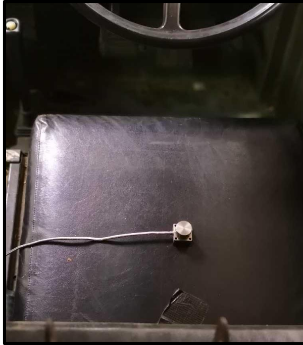
Figure 6.2 Photograph of the mounted accelerometer on the driver seat to measure the acceleration at the driver seat.
