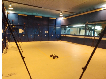
Fig. 7. Experiment set up in the flying lab at Cranfield University equipped with a VICON navigation system.
