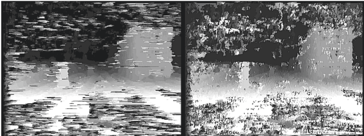
Figure 15 The raw NOMD disparity maps without refinement (left) and with refinement (right).
