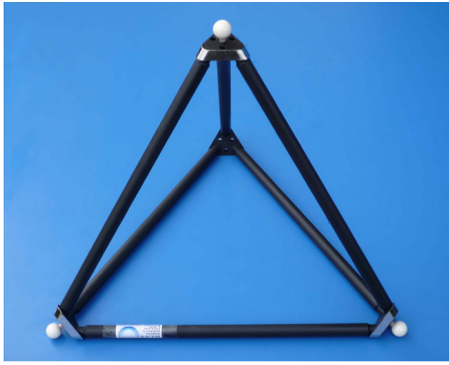
Figure 11. Carbon fibre tetrahedron artefact studied [64, 65]. Reproduced with permission from [65].
