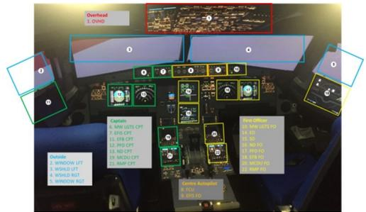
Fig. 4. Eye tracking in A320 simulator.
