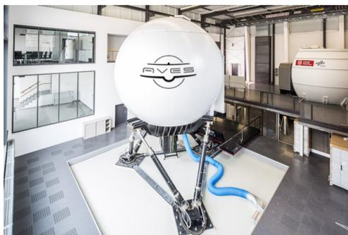
Fig. 1. The DLR AVES flight simulator.
