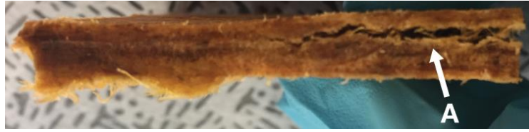
Figure 141 AK30 sample cross-section area after 2 hours of water immersion at 20 °C, delamination and fibre swelling can be observed (A)
