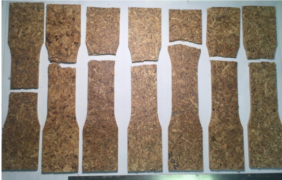
Figure_Apx 7-8 M30 control samples fractures after tensile test
