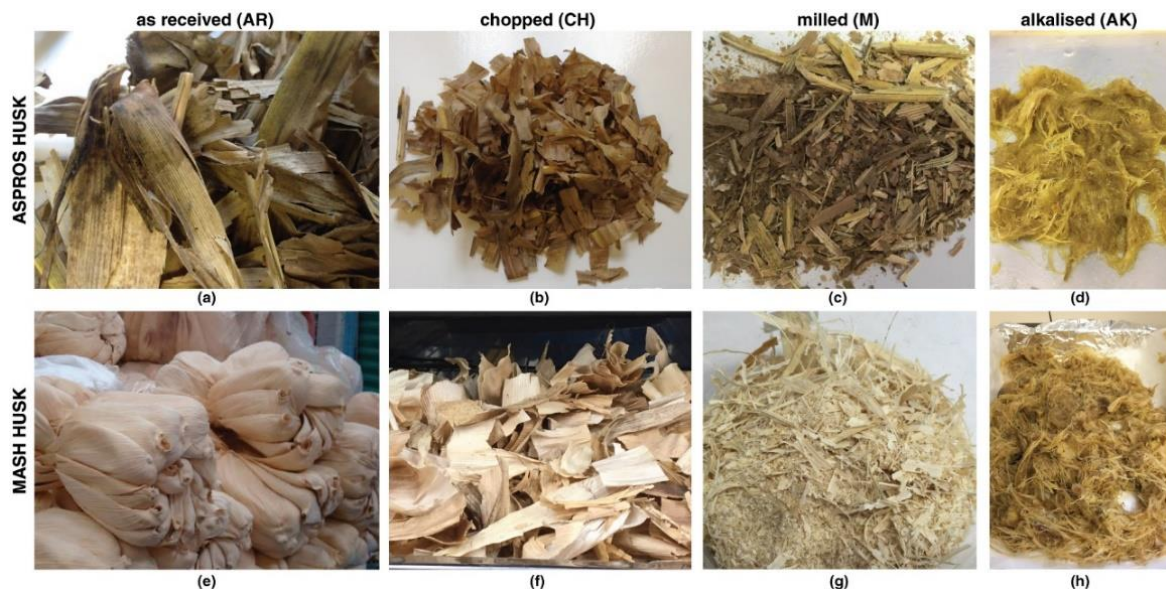
Figure 85 Husk sizes used in the MHC production, ASPROS samples are shown in the first row (a), (b), (c) and (d); and MASH samples in the row below (e), (f), (g) and (h)
