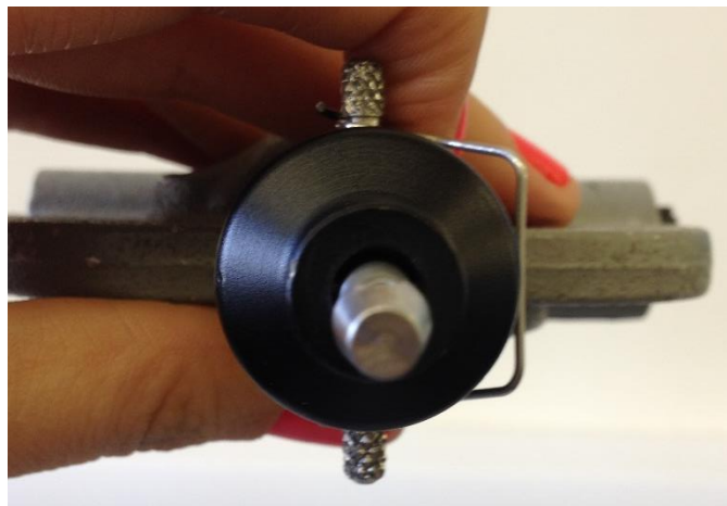
Figure_Apx 7-4 Adaptor designed for 100N load cell
