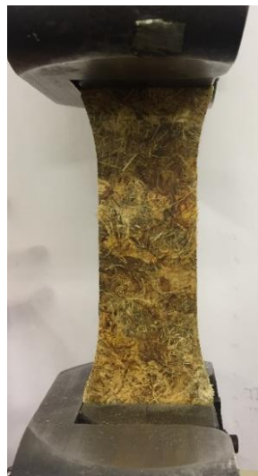
Figure 51 MHC sample placed in the testing machine for tensile test
