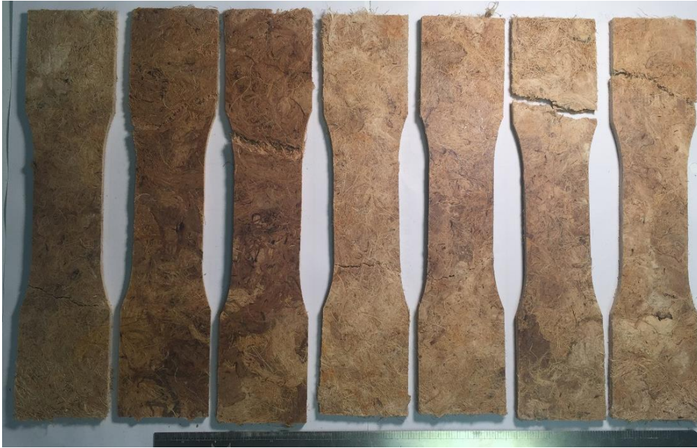
Figure 132 Aged AK30 samples fractures after tensile test
