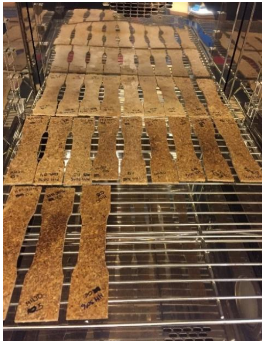
Figure 52 MHC specimens distributed in the ambience chamber
