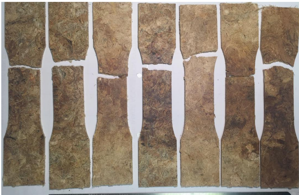
Figure 131 AK30 control samples fractures after tensile test
