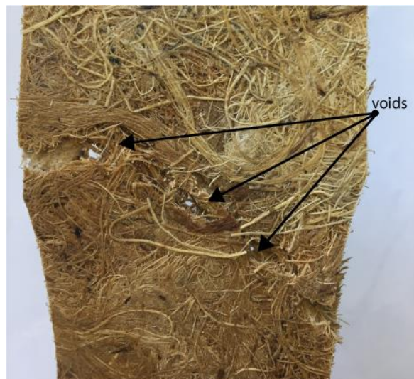
Figure 121 AK30 sample showing voids and uneven surface
