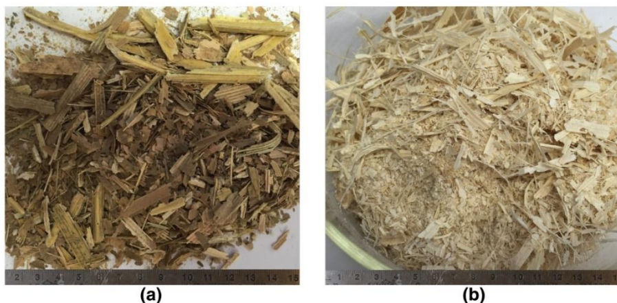
Figure 71 Milled MH batches (a) ASPROS, and (b) MASH after going through the milling process for 10 minutes at medium speed (25,000 RPM)
