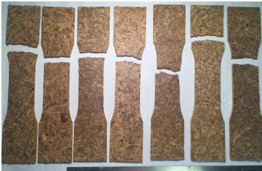
Figure_Apx 7-9 M30 aged samples fractures after tensile test
