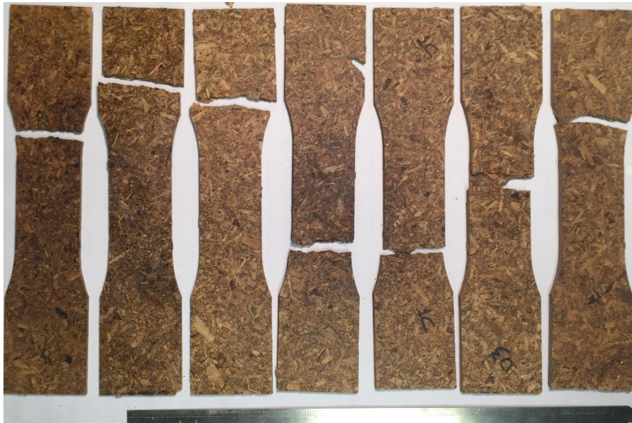
Figure_Apx 7-11 M30 aged samples fractures after tensile test
