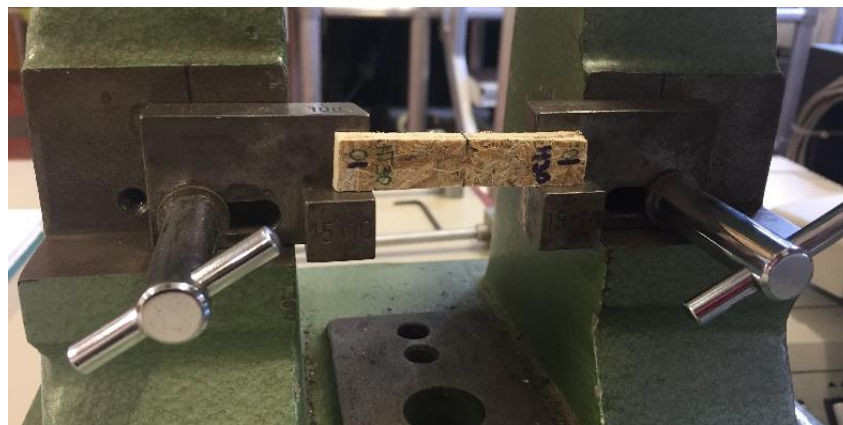
Figure 53 MHC sample placed in the pendulum for impact test
