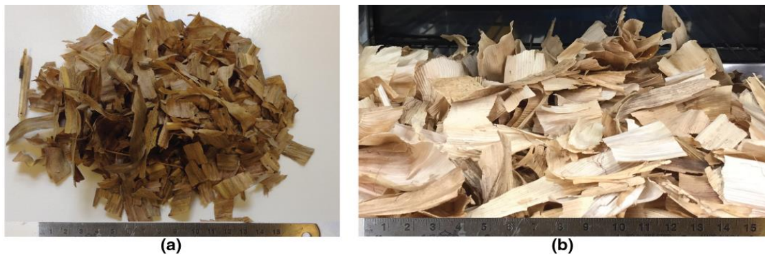
Figure 69 Chopped MH (a) ASPROS, and (b) MASH after washing; still shows a pronounced ripple shape
