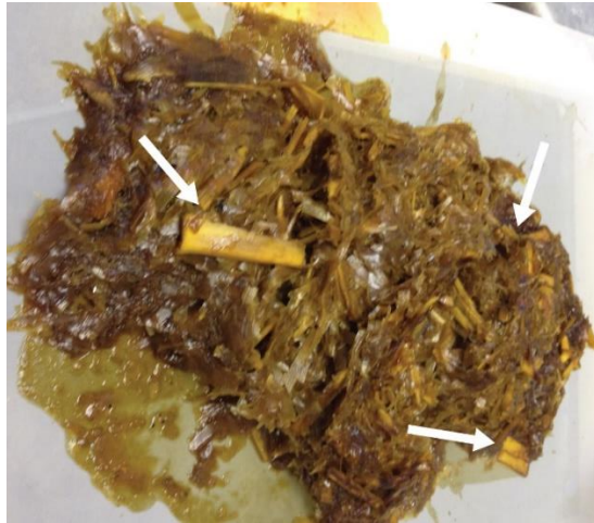
Figure 76 ASPROS husk slurry obtained from alkalinisation, showing remnants of bast structure and some fibre bundles still attached
