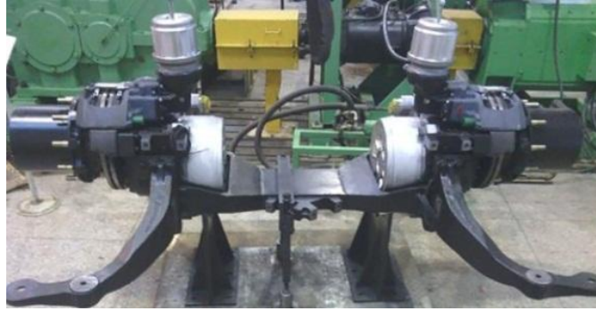
Fig. 3. Two-independent-motor driving system [51].
